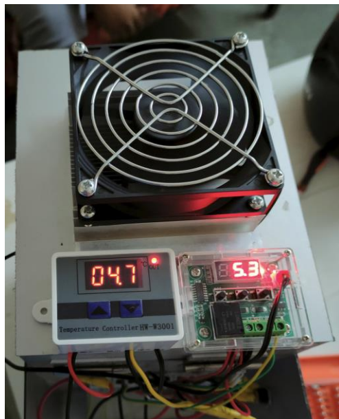
Fig 7.5 Lowest temperature reach at ambient temperature of 36°C
