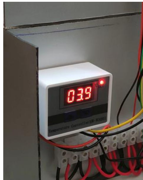
Fig 7.6 Lowest temperature reach at ambient temperature of 34°C
